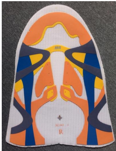
Figure 1. Mult-level Haptic coating on polyester mesh
